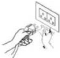
1.2 Make sure the plug is placed fully & firm into the socket!
