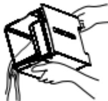
Remove the water in the water tank with two hands
